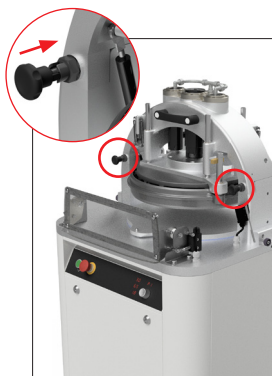
7. Close the fastening thrusts (x2)
