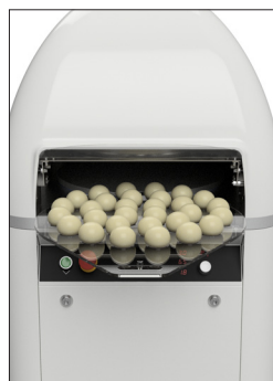
6. Open the guard casing and remove the plate with shaped balls
